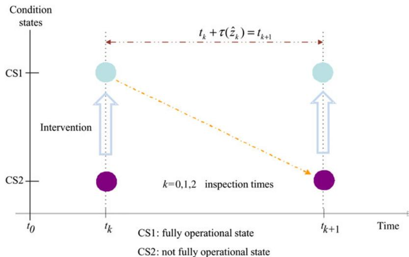
Figure 1. Deterioration and intervention process.
